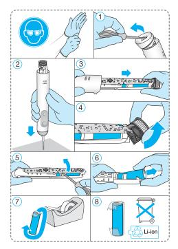
Open the handle as shown, remove the battery and dispose of it according to local environmental regulations.
