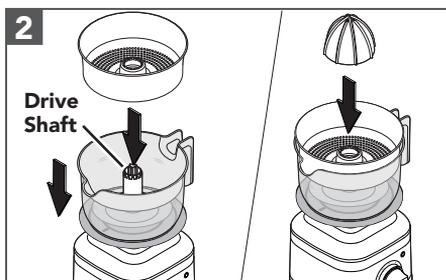
Place the Pulp Basket and then the Reamer into the Juice Container by aligning them with the Drive Shaft.
