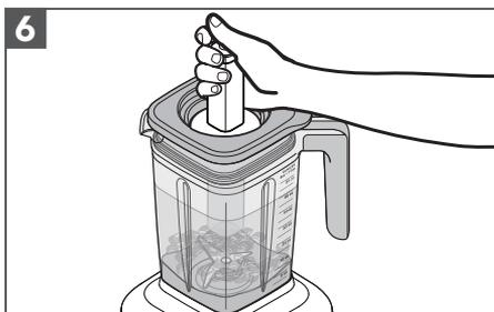
**Tamper Accessory:** Remove the Lid Centre Cap only. Stir or press contents down towards the blade. Then, place the Lid Centre Cap back before resuming blending.
