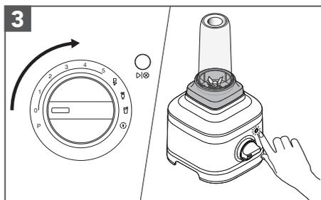
Turn from (0) to desired speed or preset recipe programme. Press (▶▶) to start. See “Blender Function Guide” for more details.
