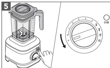
**Pulse Mode:** Press (▷|⊙). Turn and hold the Control Dial from (O) to (P) as per desired interval of time.
