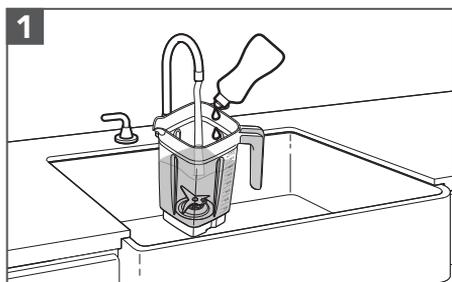
Fill half of the Jar with warm water and add 1 or 2 drops of dish-washing liquid. Place the Jar on the Base. Secure the Lid and Lid Centre Cap.
