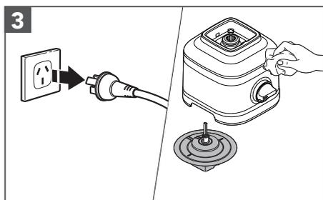
Unplug the Blender before cleaning. Wipe clean the Base, Power Cord and the Gear Assembly of the Citrus Press with a warm, damp cloth and dry with a soft cloth.
