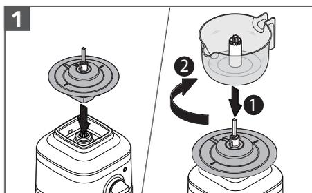
Place the Gear Assembly on Base. Place the Juice Container on the Gear Assembly and twist clockwise to lock in place.
