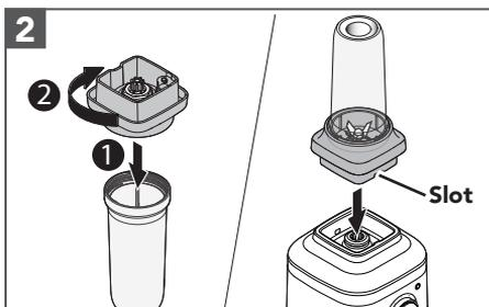
Secure the Blade Assembly on the Jar and rotate it clockwise until it is tight. Place it on the Base.
