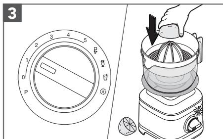
Turn from (0) to speed 1 or 2. Hold down the halved citrus fruit on the Reamer. Press (▶▶) to start.
